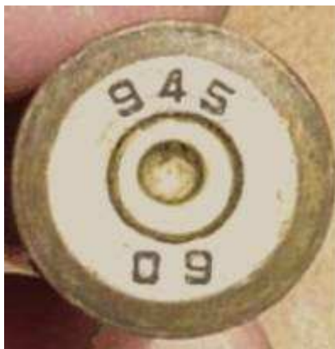
On the left, a box of ammunition captured from SAF in South Kordofan in July 2011. All rounds of ammunition bear identical marking-codes (company code '945' and year of manufacturing code '09'); and on the right, a 7.62x54mm cartridge collected in Darfur in mid-2010 by the UN Panel of Experts on the Sudan (see S/2011/11). The headstamp bears the company code '945' and year of manufacturing code '09' as in 2009. © Private.
